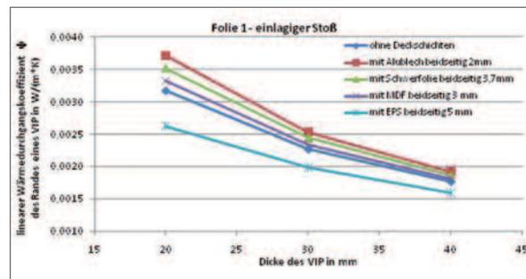
Linear thermal transmittance of panel edge of VIPs with various cover materials
