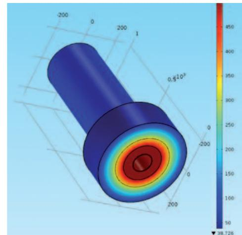
Figure 2: Insulated flange in finite element analysis
