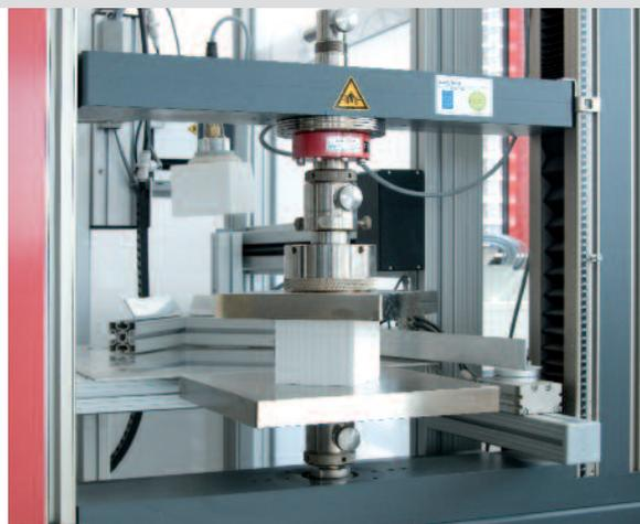
Automation of the compressive test
