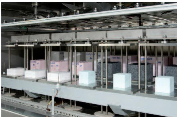
Samples in an oven for the determination of the deformation under temperature and load
