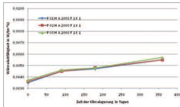
Long-term increase of thermal conductivity for temperature storage of VIPs
