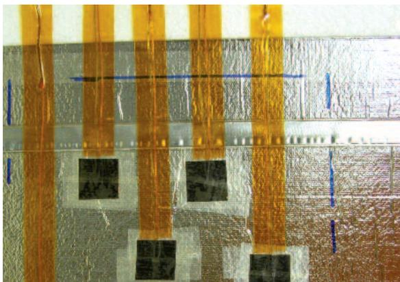
Measurement of thermal conductivity of VIP
