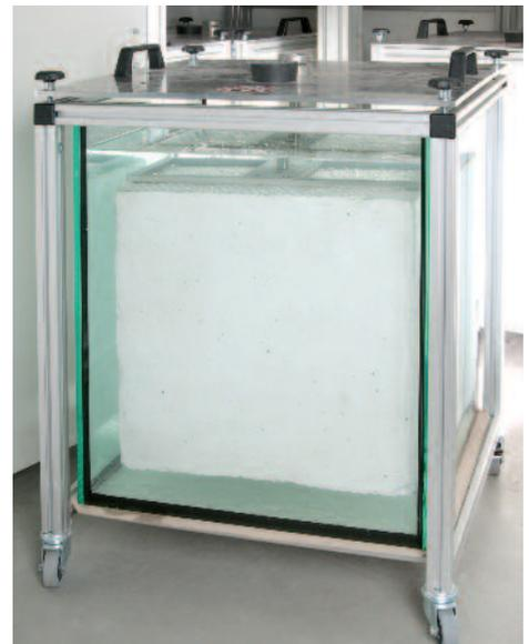
Water absorption of EPS with high thickness
