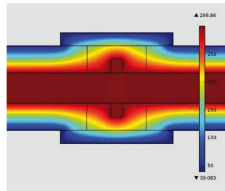
† temperature curve of a FEM-simulation for a flange cap according to the state of technology
