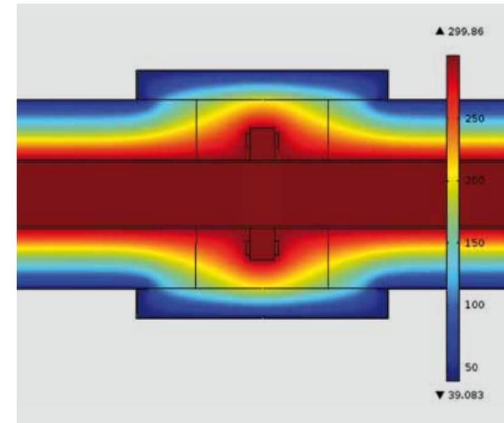
† temperature curve of a FEM-simulation for a flange cap according to the state of technology
