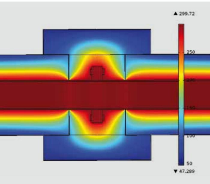
† temperature curve of a FEM-simulation for a best-practice flange cap
