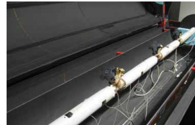
from the beginning to the end of the measurement section. On the other, a heat flow meter is installed whose signal is proportional to the measuring system's heat loss. An additional test only with the pipe insulation provides the heat loss via the insulation.
