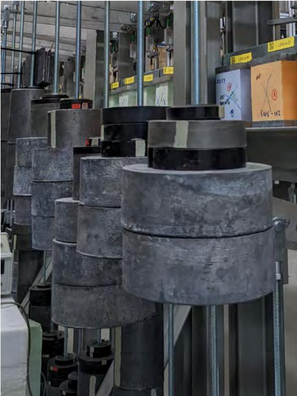
Long-term creep: in some cases large weights on the lever to simulate the substantial load of a building
