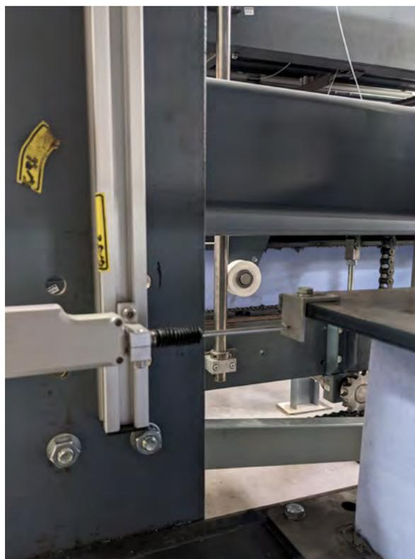
**Adopted testing device** for determining long-term creep behaviour with shear effect and new FIW measuring technique
