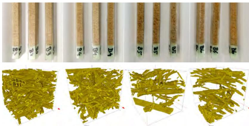
**Fig. 1 above:** Sample preparation of wood fibre insulation materials of different densities (FIW); **below:** volume rendering of the variants B3 - B6 based on high-resolution tomographic images (ITWM)
