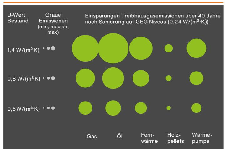
**Fig. 2:** Comparison of expense to achievable GHG savings over 40 years for refurbishment to a U-value of 0.24 W/(m²·K) for various existing buildings
