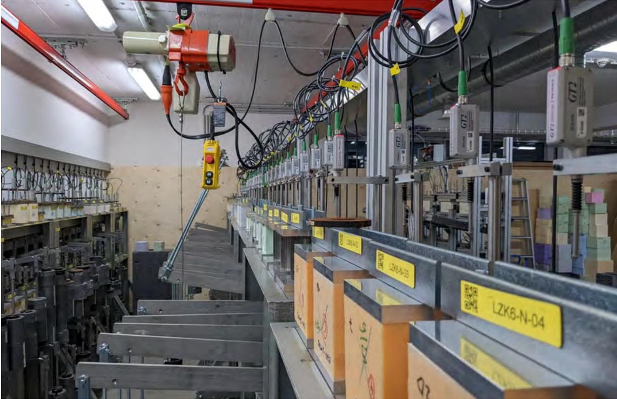
Determining long-term creep behaviour, new test stands with variable sample size
