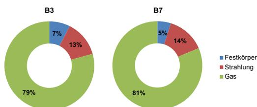
**Fig. 4:** Results of the proportions of the heat transfer mechanisms for two variants
