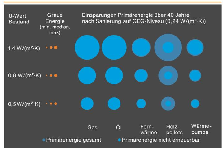
**Fig. 1:** Comparison of expense to achievable savings in total and non-renewable primary energy over 40 years for refurbishment to a U-value of 0.24 W/(m²·K) for various existing buildings
