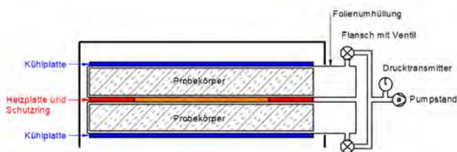
**Fig. 3:** Schematic diagram of the experimental set-up for determining the proportions of the heat transfer mechanisms
