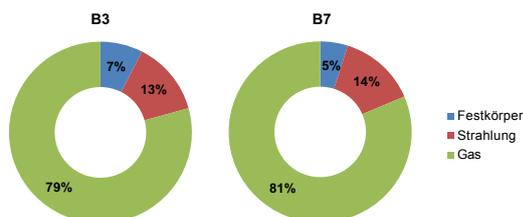
**Fig. 4:** Results of the proportions of the heat transfer mechanisms for two variants
