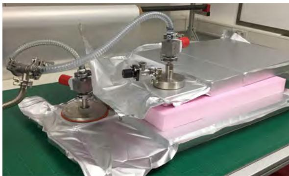
**Fig. 2:** Test specimen for determining the proportions of the heat transfer mechanisms with foil wrapping and flanged evacuation adapter
